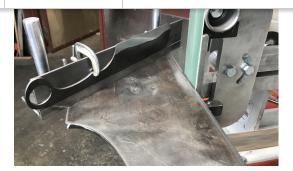
grinder, and a knife grinding jig.
